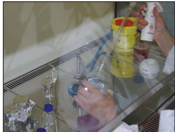
Figure 62. All operations should be performed in a sterile laminar flow unit
