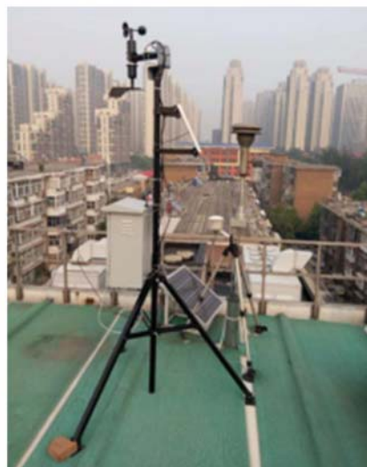
The multi-parameter outdoor air quality monitor
