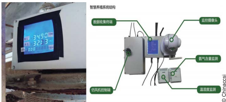
Multi-parameter environmental monitor for intelligent animal husbandry
