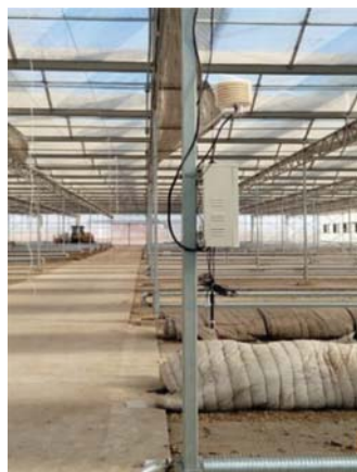
Multi-parameter farming environment monitor
