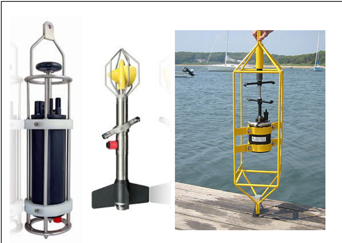
Figure 4: Example discrete current meters. L to r: electromagnetic current meter (ECM), impeller-type meter, acoustic-type meter.
