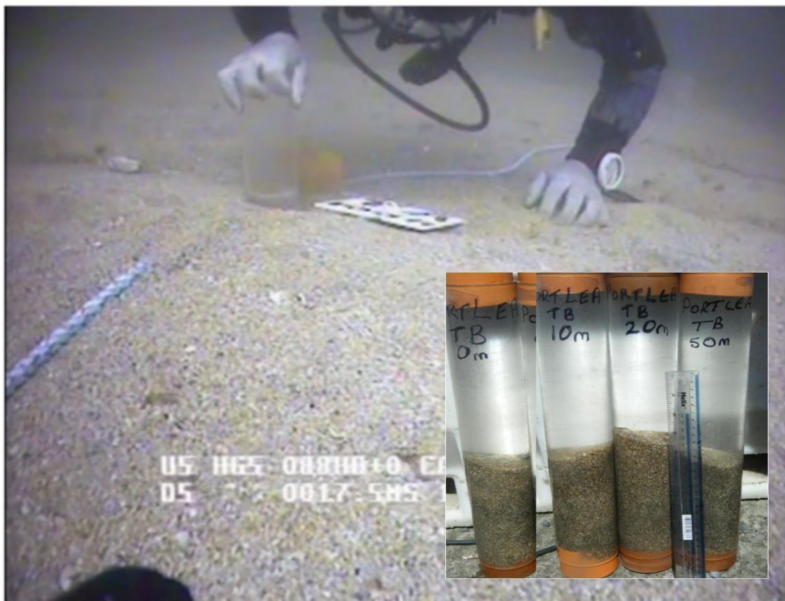
Figure 12: Videographic survey still, showing deployment of corer into the sediment. Corer is a plastic tube of known diameter (approx 4-5cm) pushed into the sediment by hand. Retrieved cores (inset). Courtesy and copyright of marine harvest Ireland.
