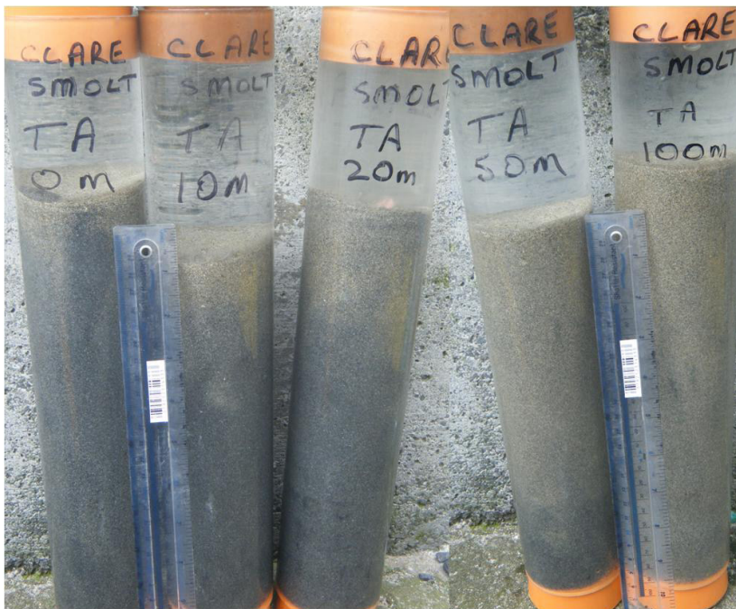
Figure 3: Core samples from [site name] fish farm site taken along Transect A at 0 m, 10 m, 20 m and 100 m from cage edge.
