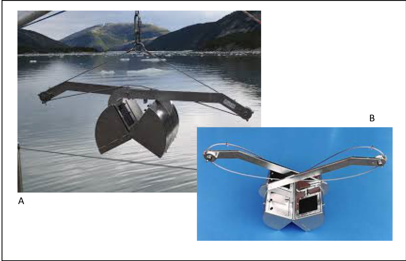
FIGURE 13: VAN VEEN GRAB SAMPLER, FOR SEDIMENT COLLECTION IN DEPLOYMENT MODE (A) AND IN CLOSE-UP TO SHOW TOP OPENINGS FOR PHYSIO-CHEMICAL SAMPLE COLLECTION (B). ILLUSTRATIVE PURPOSES ONLY AND OTHER TYPES ARE AVAILABLE. SIZES USED GENERALLY 0.025 M 2 , 0.045 M 2 OR 0.1 M 2 .
