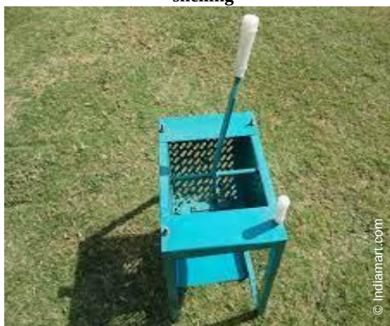
Figure 60. Megakonnnect hand operated Groundnut Decorticator is small machine for shelling
