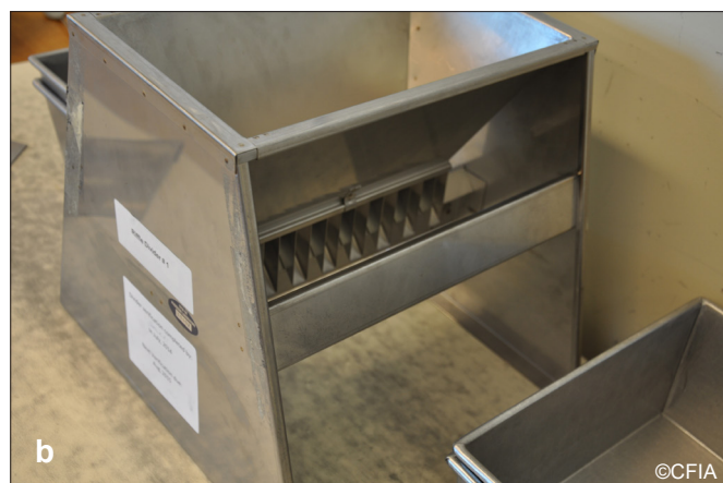
Figure 7.2. Soil (riffle) dividers: a non-tipping type (left) and tipping type (right); b detail of non-tipping type riffle divider (images courtesy of ISTA accredited laboratory CA08)
