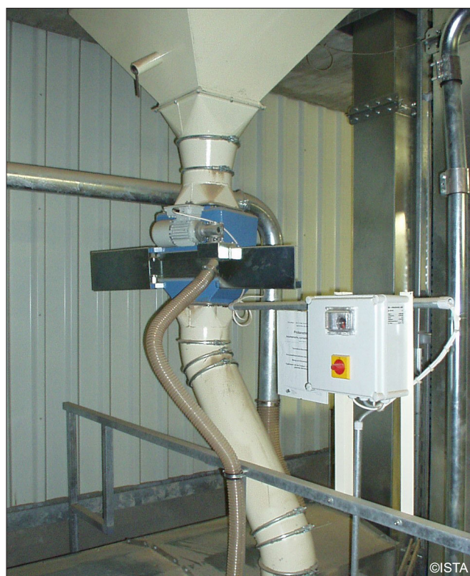
Figure 6.5. An automatic sampler of the moving beak type, with the collection of a composite sample into a plastic tube (image courtesy of ISTA)
