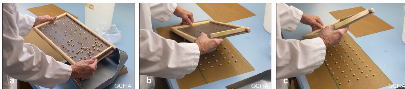
Figure 8.13. Using a counting board: a filling the seed into the 50 holes and removing the excess seeds; b lifting the board away from the pre-wetted paper towel after the seeds have been released by pulling back the lower part of the board and allowing the seeds to remain on the towel; c the 50 seeds are evenly spaced on the single layer of wet paper towel ready to have another layer of wet paper added on top, before folding and rolling to complete preparation of one of eight replicates of 50 seeds for a 400-seed germination test (images courtesy of ISTA accredited laboratory CA08)
