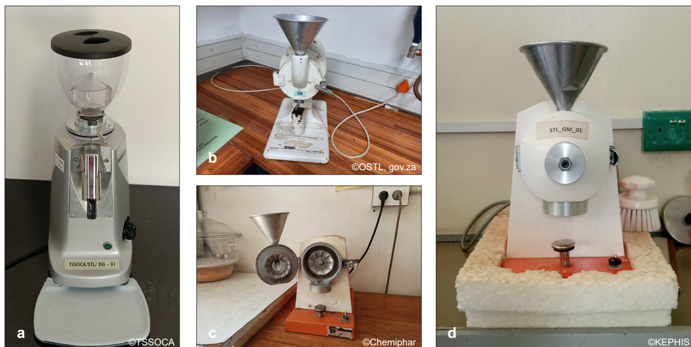
Figure 10.4. Grinders for preparation of seed moisture samples: a disc grinder; b adjustable coarse and fine grinder; c–d seed grinders (images courtesy of ISTA accredited laboratories IN39, ZA01, UG02 and KE01)
