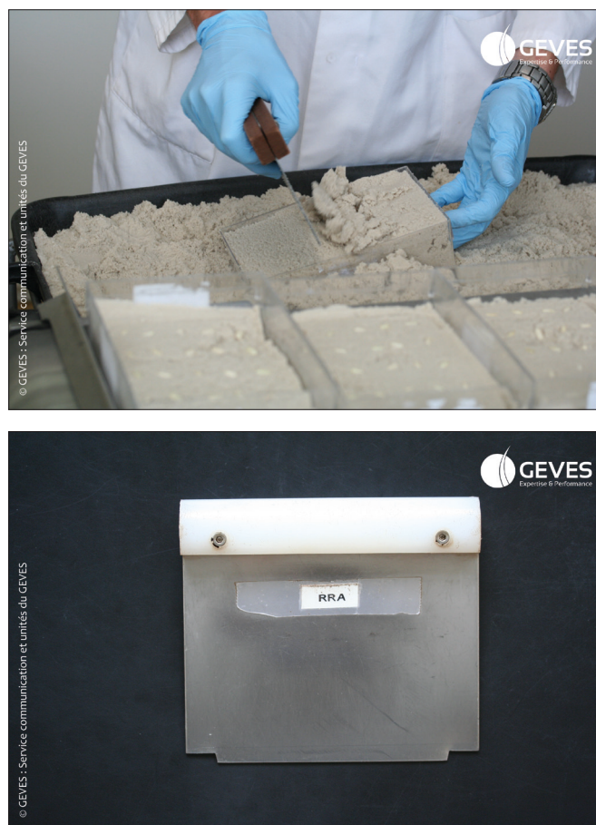
Figure 8.15. Use of a scraper (detail, bottom) to ensure a constant layer of substrate (images courtesy of ISTA accredited laboratory FR02)
