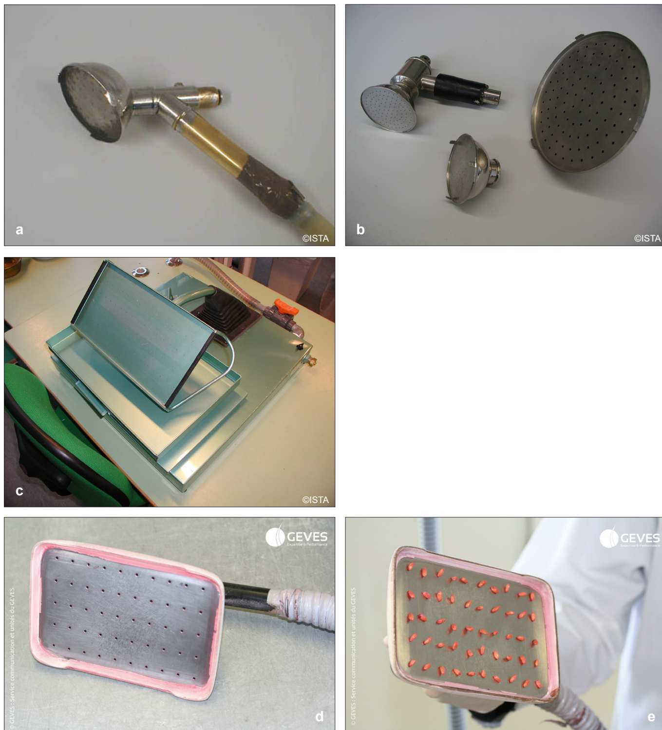
Figure 8.12. Vacuum counting heads: a typical head for planting; b various heads for different sizes of seeds and blotters; c vacuum planter for cereals; d head with large-sized holes for cereal seeds; e head with seeds attached (images a–c courtesy of ISTA; images d and e courtesy of ISTA accredited laboratory FR02)
