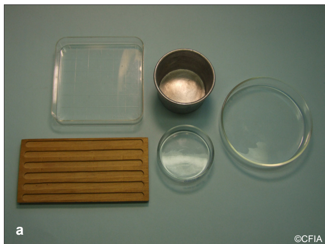
Figure 7.9. Containers for purity analysis and other seed determination: a beakers, glass, metal and a wooden tray; b larger containers (images courtesy of ISTA accredited laboratory CA08)
