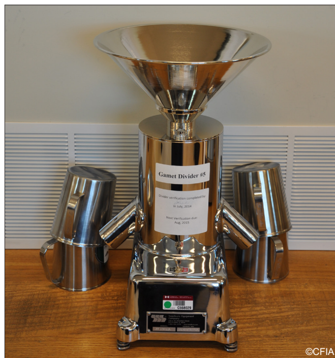
Figure 7.3. Gamet type centrifugal divider (image courtesy of ISTA accredited laboratory CA08)
