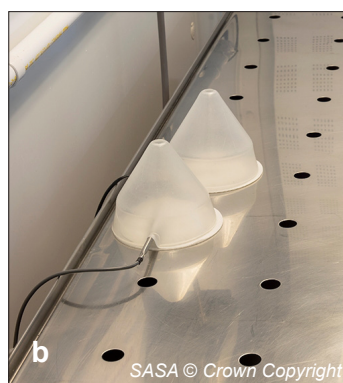
Figure 8.9. a Bell jars to prevent tests drying out on a germination table; b with temperature probe (images courtesy of ISTA accredited laboratory GB04)
