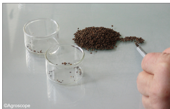
Figure 7.12. Analytical purity tests showing the three fractions produced (pure seed, other seeds and inert matter) for Sorghum bicolor subsp. drummondii (a) and treated Zea mays (b) (images courtesy of ISTA accredited laboratory RO05)
