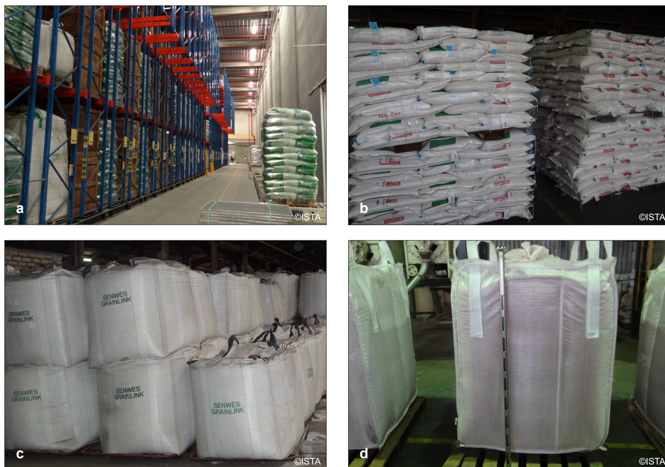
Figure 6.2. Seed storage in a warehouse: a grass seed warehouse, Denmark; b pallets stacked with 25 kg bags; c large bags stacked; d large bag and double-sleeved sampling stick (images courtesy of ISTA)
