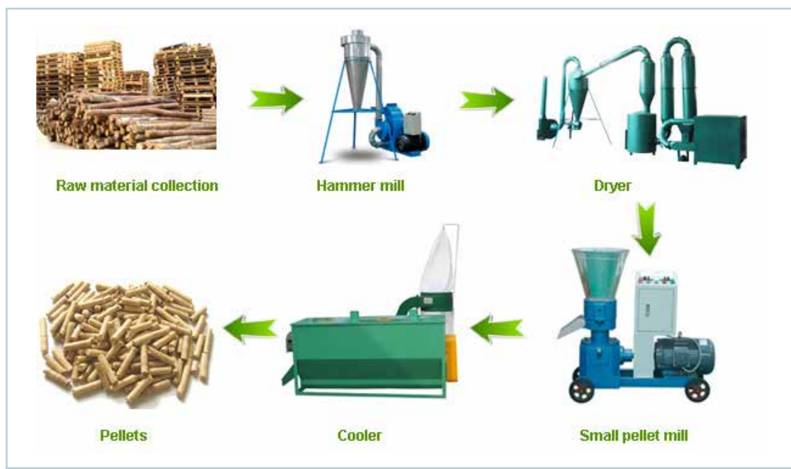
► FIGURE 19 Overview of pelletizing process
