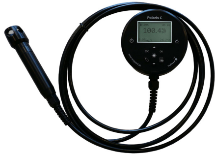
Figure 5.7 Handy Polaris oxygen metre for measuring oxygen content of the water in mg/L and % saturation
