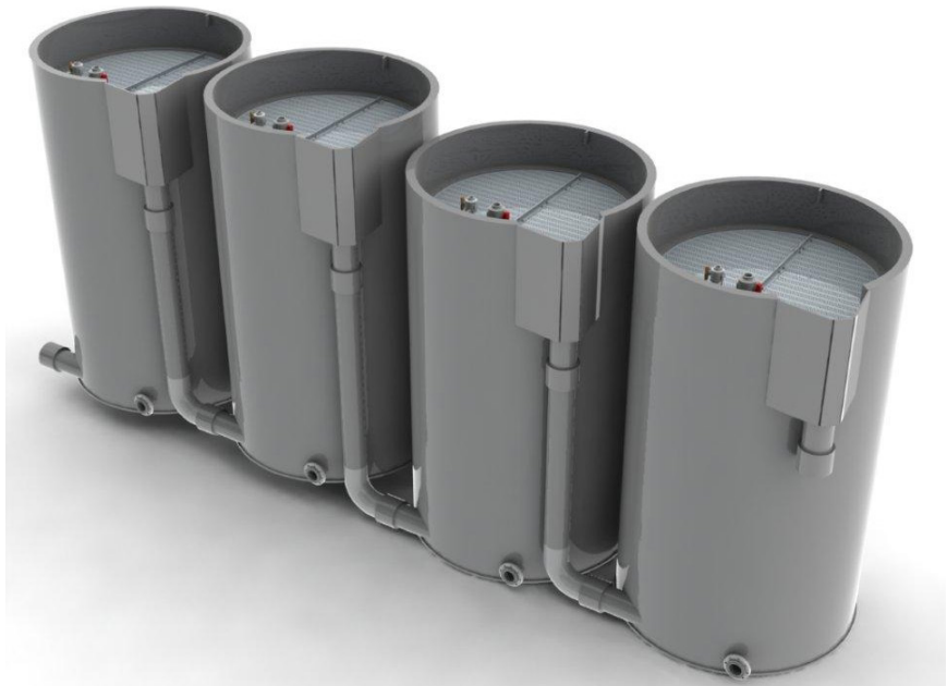
Figure 5.5 The flow pattern in the shown multi chamber PE biofilter goes from left to right and upstream in each chamber
