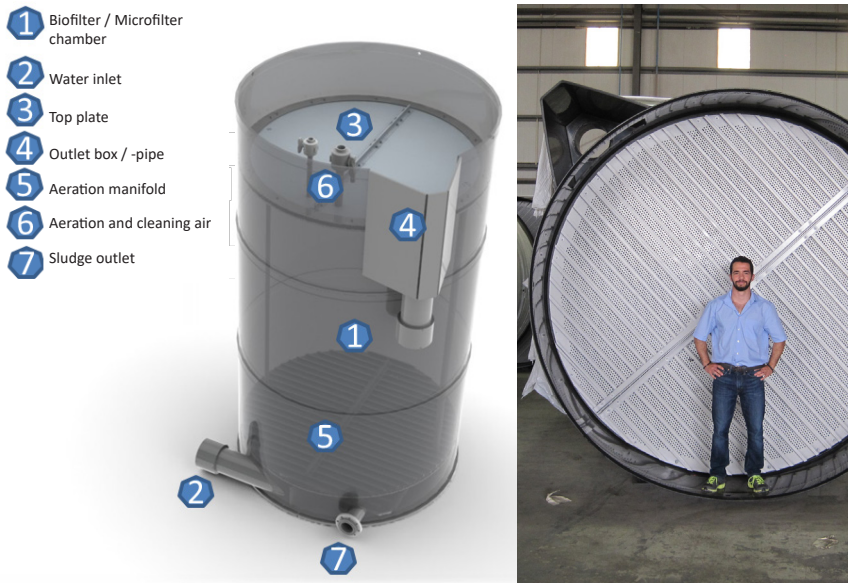
Figure 5.4 Principle drawing of pre-fabricated biofilter made of polyethylene (PE)
