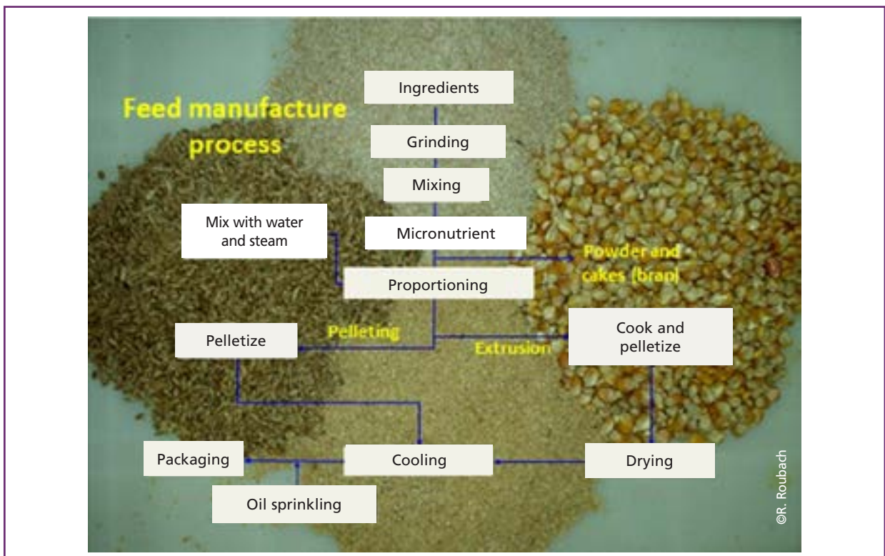
Figure 34: Feed manufacturing process
