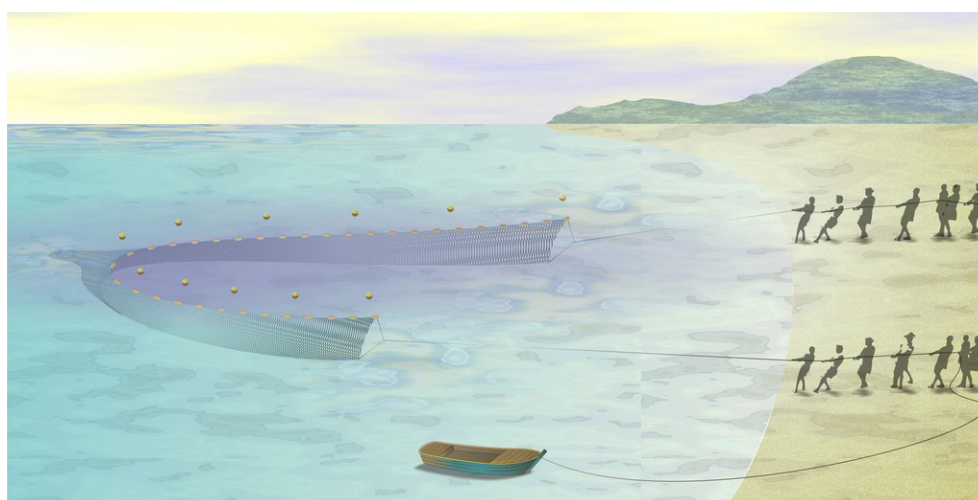
FIGURE 6 Beach seine (SB 02.1) with a codend, pulled by hand to the beach
