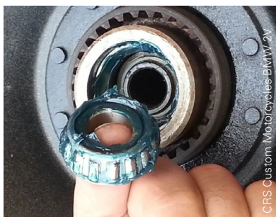
Figure 6: Lubricating bearings with multipurpose grease, and a wall bearing with oil pump used for lubrication of inner components
