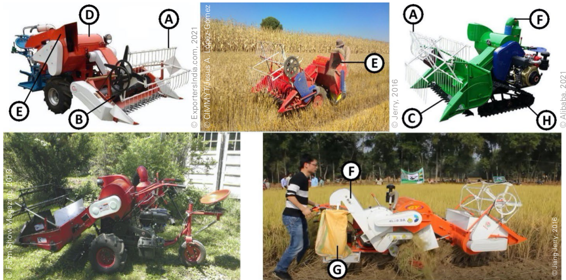
Figure 67: Small-scale self-propelled combine harvester options and its components, with (A) revolving reel, (B) intake auger or worm screw, (C) cutter bar, (D) thresher drum, (E) straw material outlet funnel, (F) grain collector tube and (G) collecting bags for clean grain. Note the option with (H) tracks, instead of tires on the green harvester on the right, which facilitates movements on mulchy terrains.
