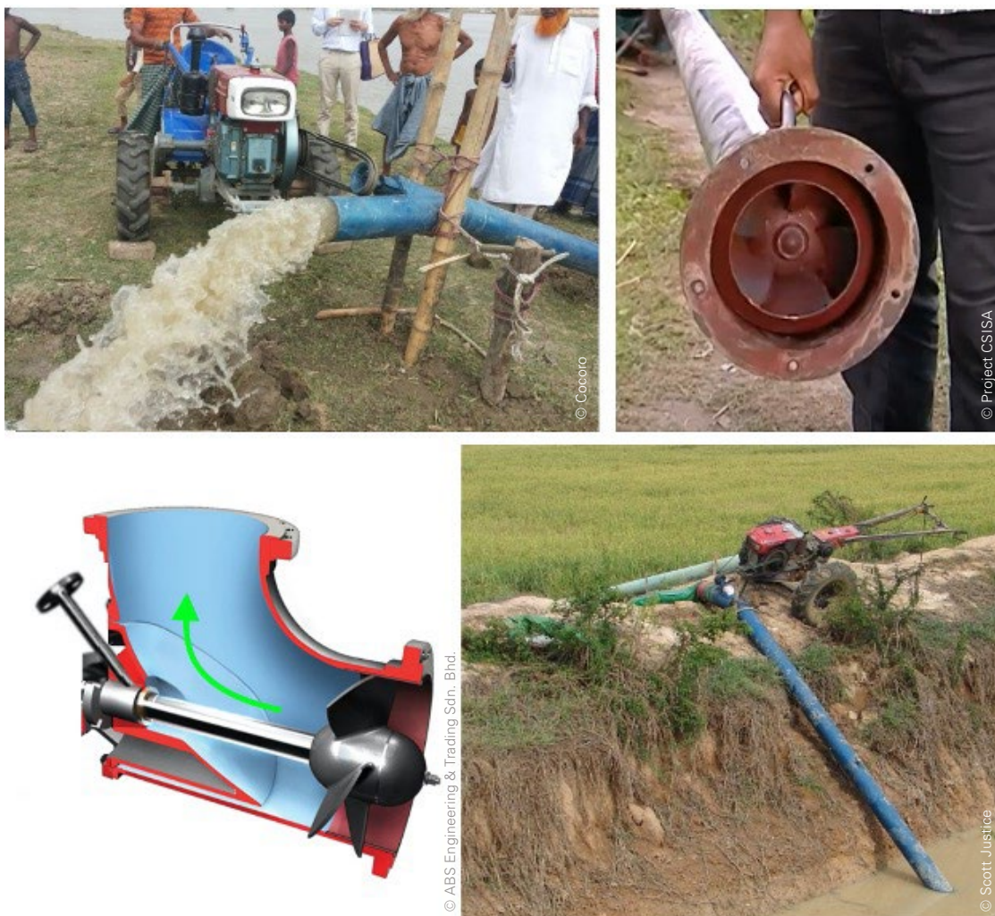
Figure 61: Axial flow pump rigged to a two-wheel tractor using the v-belts, with a close-up of the propeller sucking up the water and diagram of the pump's internal mechanism
