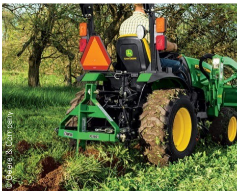
Figure 38: Levelling scraper knife manually controlled by means of the tractors' hydraulics (left) and laser land leveller with automated mechanism (right)
