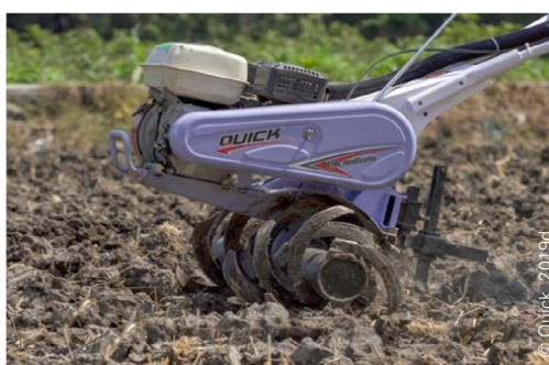
Figure 27: Small petrol 2WT with the standard farm tires (left) and a similar machine with tires replaced with blade rollers for tillage
