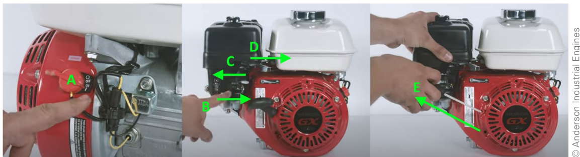
Figure 21: Starting a 2WT petrol engine, by turning on the switch button (A), opening fuel (B), closing the choke (C) and opening throttle (D), ready to crank start by pulling the ignition cord (E).
