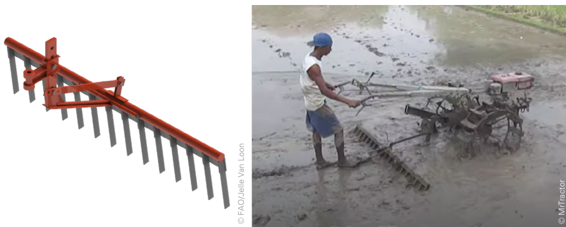
Figure 47: Wet paddy field leveller to smoothen and loosen the top mud-layer before transplanting (right)
