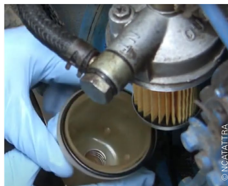
Figure 12: Fuel filter and fuel valve on tractor in OFF position to replace the filter (left) and replacement of paper fuel filter after cleaning the housing and replacing the O-ring (right).
