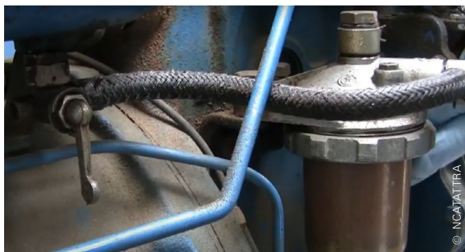
Figure 12: Fuel filter and fuel valve on tractor in OFF position to replace the filter (left) and replacement of paper fuel filter after cleaning the housing and replacing the O-ring (right).
