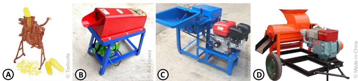
Figure 74: Manual maize table sheller (A), electric single cob maize sheller (B), petrol engine dual cob maize sheller (C) and a diesel-engine powered maize sheller trailer (D).
