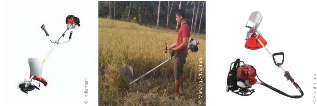
Figure 69: Portable motorized cutter implements as an intermediate solution to mechanize harvest in cereal crops, with a hand-held version on the left and centre, and a back-pack carried version on the right. Notice how both models present a shield to gather the cut-off material to one side during operation.
