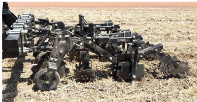
Figure 37: A chisel plow (upper – left) and right and strip-till implement (lower), performing vertical tillage to provide grooves for water infiltration and loosen up hardened soil for direct seeding, cutting through the crop residue.
