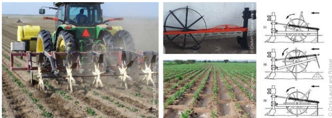
Figure 43: A rotary dammer-diker punching water harvesting holes in the furrow (left), and shovel type dammer-diker unit that can be attached on a frame to create rectangular shaped water pockets
