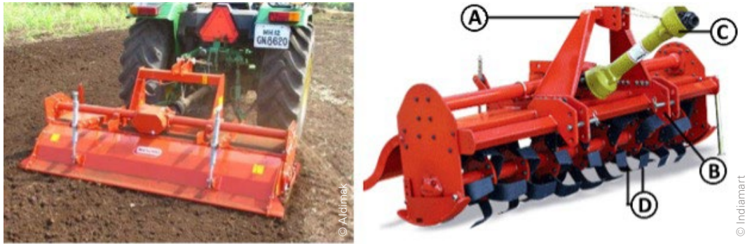
Figure 44: A rotavator attachment pulverizing the soil as secondary tillage, with main components, namely (A) central hitch tower, (B) lateral hitch pint, (C) PTO connecting rod, and (D) C-shaped rotavator blades
