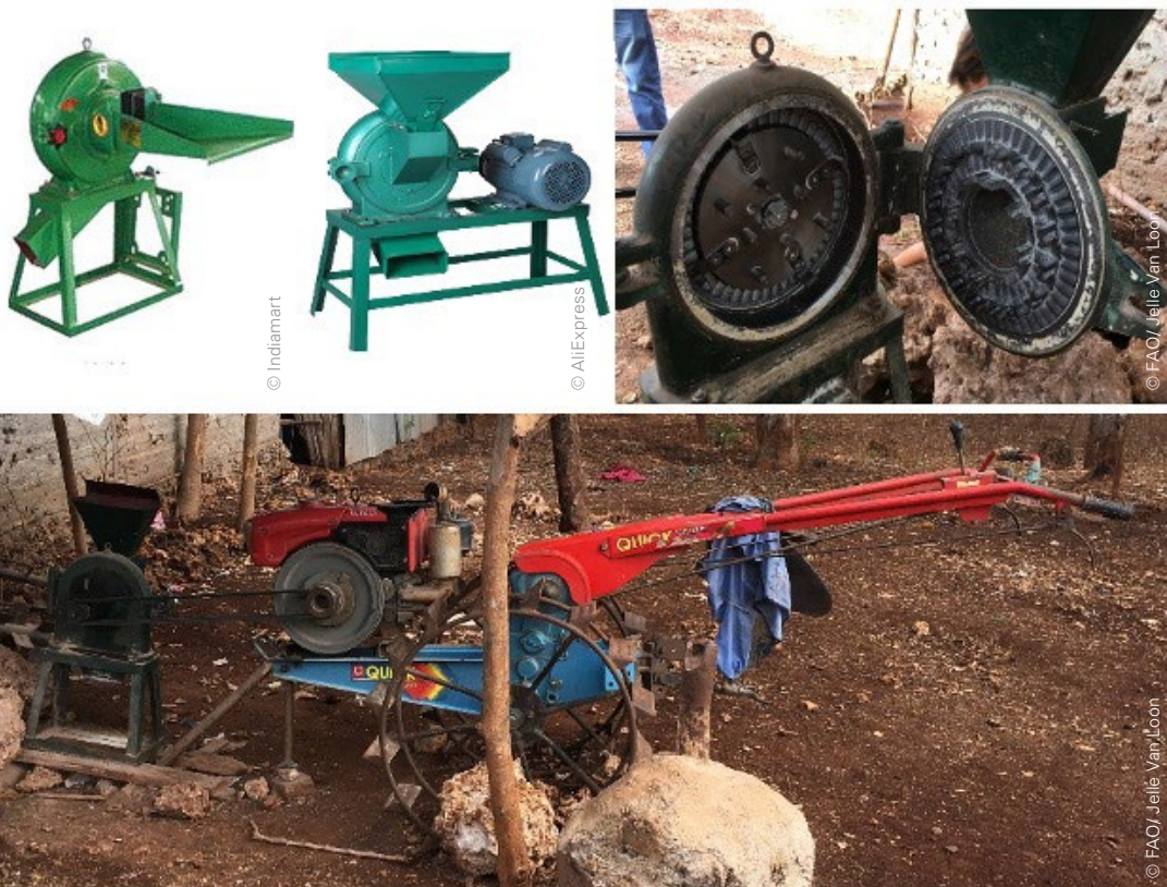
Figure 76: Overview of hammer-type maize mills (upper left), with an electric engine in the upper centre, an inside view on the upper right and below, attached to and powered by a two-wheel tractor at a farmers' homestead.
