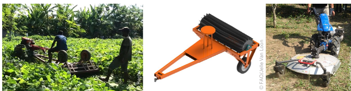
Figure 48: Two-wheel tractor operated roller-crimper (left) and small brush shredder/mover frontally attached to the PTO of a petrol engine 2WT (right)
