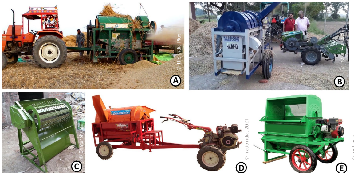
Figure 73: Different thresher machinery, with (A) tractor-pulled mobile thresher trailer, (B) two-wheel tractor powered rice thresher, (C) a human-powered pedal thresher, (D) a two-wheel trailed thresher and (E) a self-propelled pushcart model.
