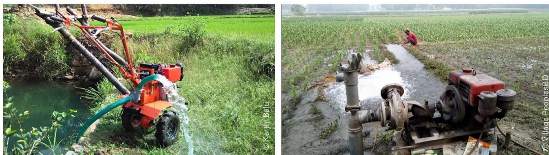
Figure 62: Radial flow pump attached to PTO of a small petrol-engine 2WT (left) and attached directly to the flywheel of a diesel engine 2WT (right)
