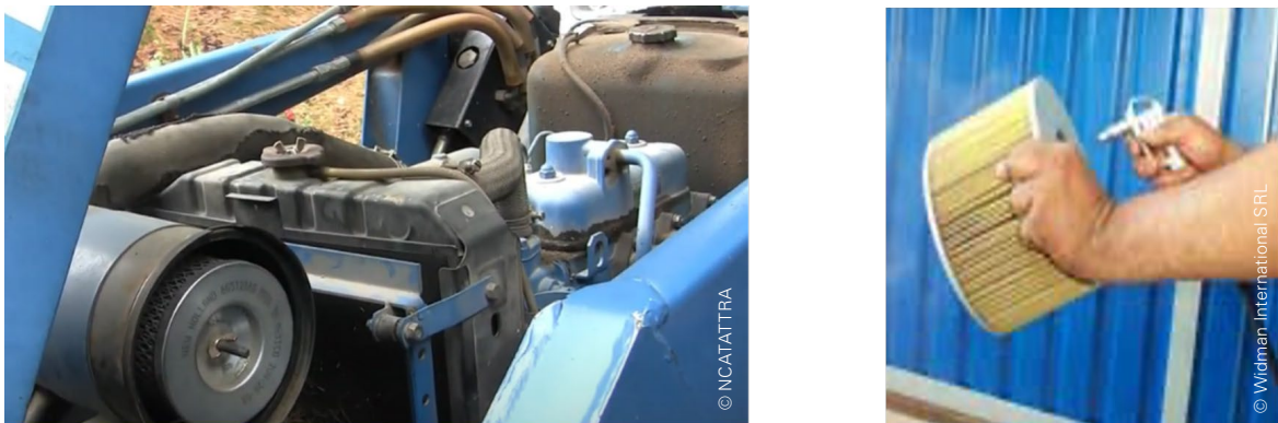
Figure 11: Cylinder-shaped air filter located in front of tractor radiator and cleaning of air filter with compressed air from inside out and at a distance.
