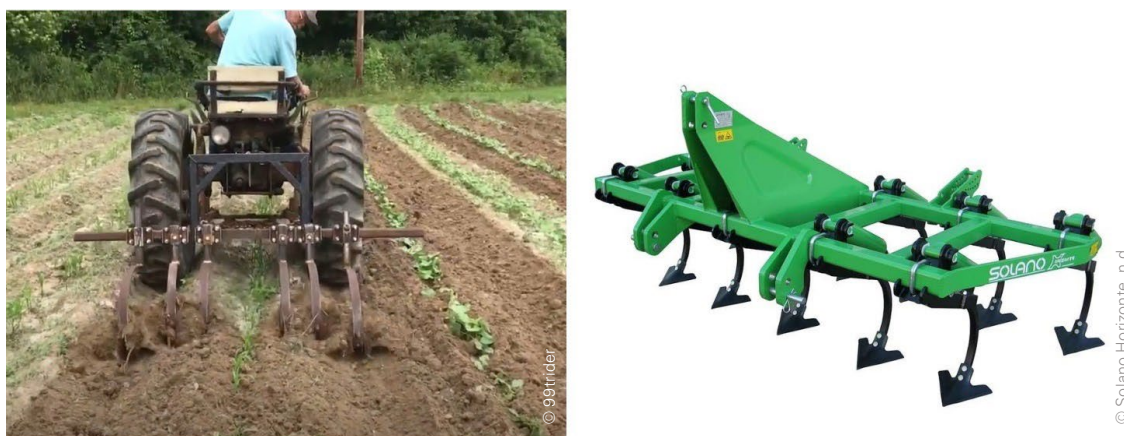
Figure 63: Four-wheel tractor pulling a homemade cultivator to control weeds in the field during crop growth (left), and cultivator machine with triangular cultivator tines/scrapers (right)
