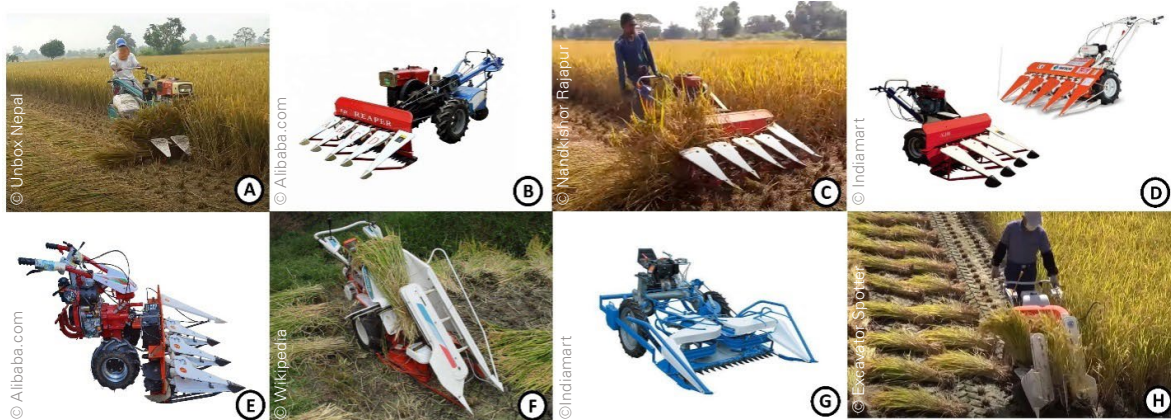
Figure 66: Different types of reaper equipment and its operation in the field (A) and (B), two-wheel tractor reapers (C) and (D), self-propelled petrol engine reapers (E) and (F), and reaper-binders (G) and (H)
