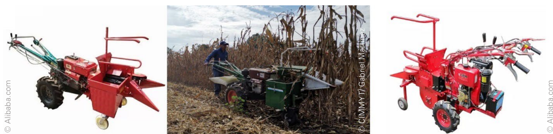
Figure 68: Small-scale single line maize harvester type, with a two-wheel tractor version on the left and a self-propelled version on the right
