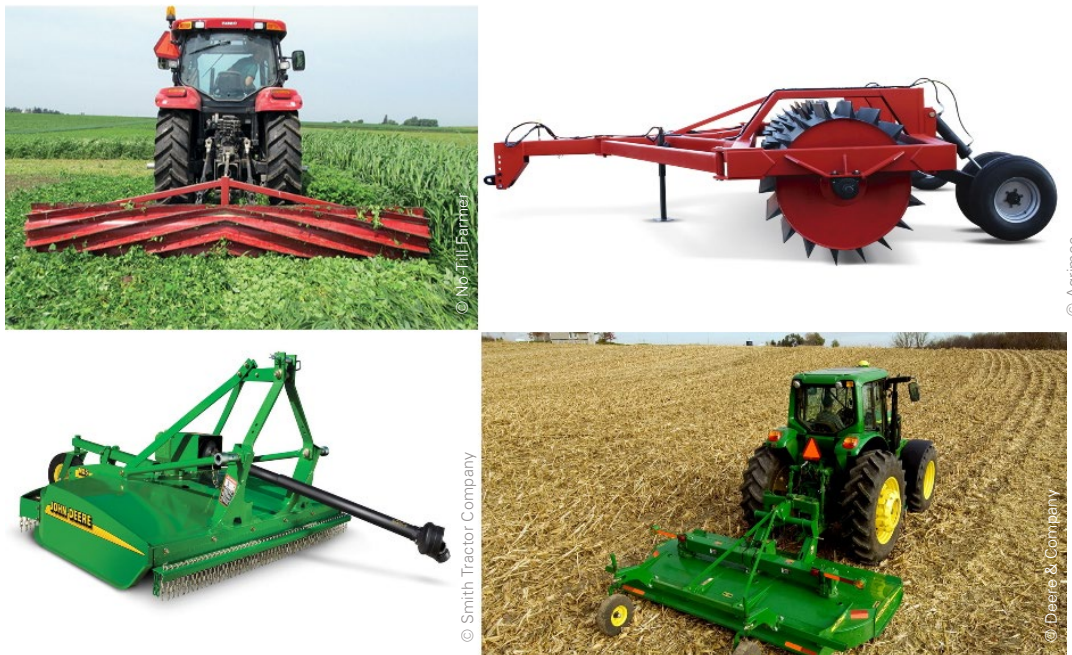
Figure 41: A knife-roller or roller-crimper being pulled by a tractor crushing the vegetation (upper left and right) and a horizontal shredder/mover trimming maize stubble spreading the crop residue evenly over the field (bottom left and right)
