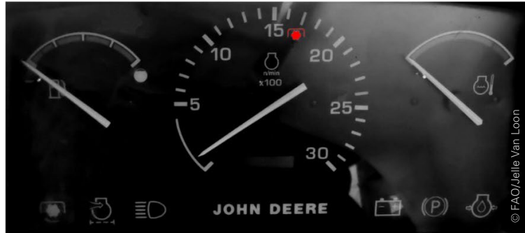
Figure 3: Standard power take-off (PTO) shaft or cardan with flexible end joints, and diagram of tractor dashboard with an indicator light that shows optimal engine RPM to use the PTO marked in red Note: Engine revolutions, which show on the dashboard of the tractor are not the same as PTO revolutions, the symbol marked in red represents the engines revolutions at which the PTO reaches its operational velocity (either 540 or 1000 rpm, depending the model). In this case, the tractor indicates that at 2000 rpm engine revolutions the PTO reaches operational speed.
