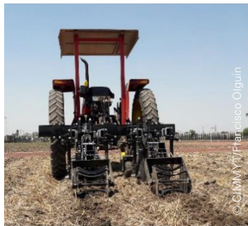
Figure 37: A chisel plow (upper – left) and right and strip-till implement (lower), performing vertical tillage to provide grooves for water infiltration and loosen up hardened soil for direct seeding, cutting through the crop residue.
