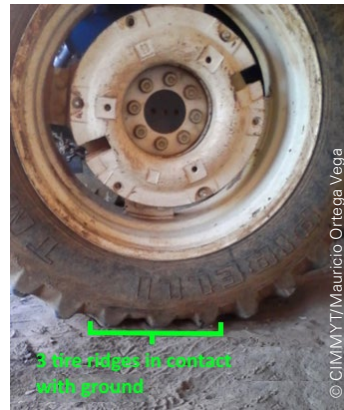
Figure 5: Diagram of checking and adjusting the tension in drive train chains using a tensioner pulley (A), level (B) and ruler (C) on the left, and correct tyre pressure with three tyre ridges in contact with the ground on the right.
