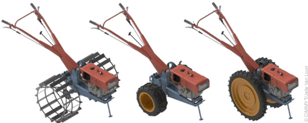
Figure 25: Different wheelsets on 2WT, with long wheel cage for deep paddy fields (left), double tires for extra traction in muddy and sloped terrain (centre), and high tires with cultivation purposes (right)
