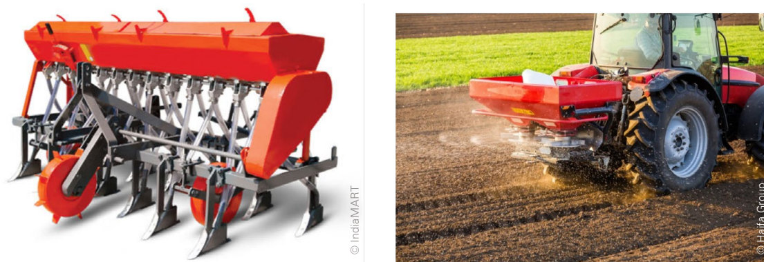
Figure 51: Generic mechanical fertilizer machine with traction provided by a spiky steel wheel rolling over the soil (left) and broadcast fertilizer application (right)
