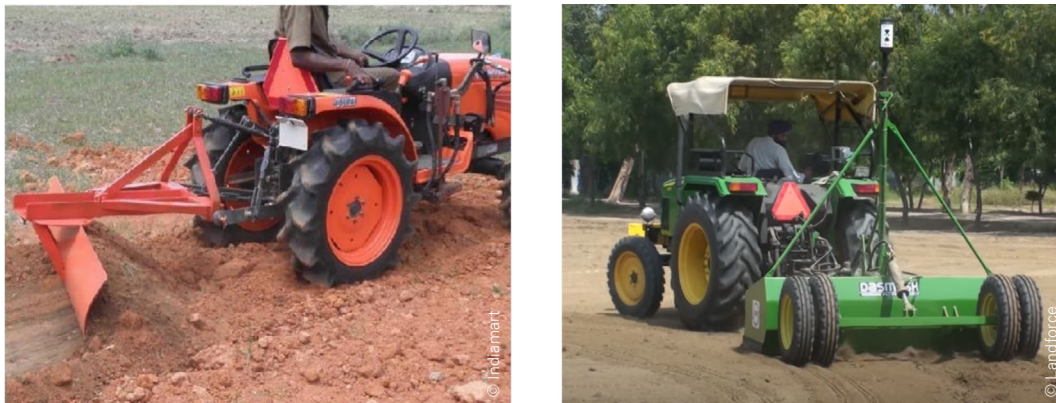
Figure 39: Levelling scraper knife manually controlled by means of the tractors' hydraulics (left) and laser land leveller with automated mechanism (right)
