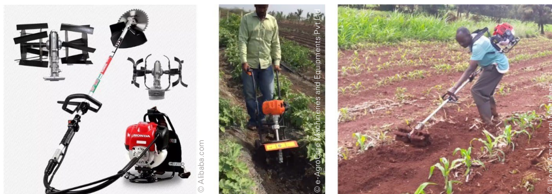
Figure 64: Examples of hand-held power weeders, with stroller and backpack system.
