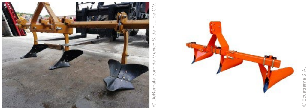
Figure 42: Two different types of ridgers; on the left, a ridger often used to create plot borders and on the right, a wing-shaped ridger more commonly used for bed-making.
