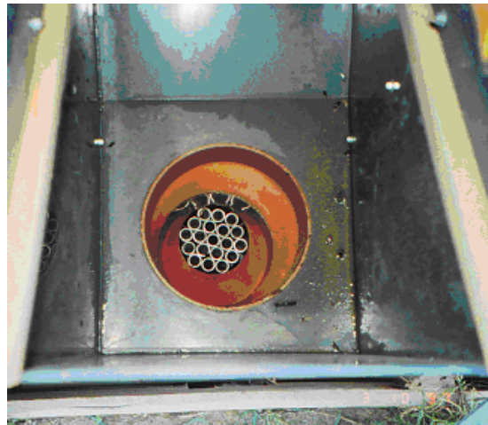
FIG. 4. Multi-tube divisor with sampling tube.
