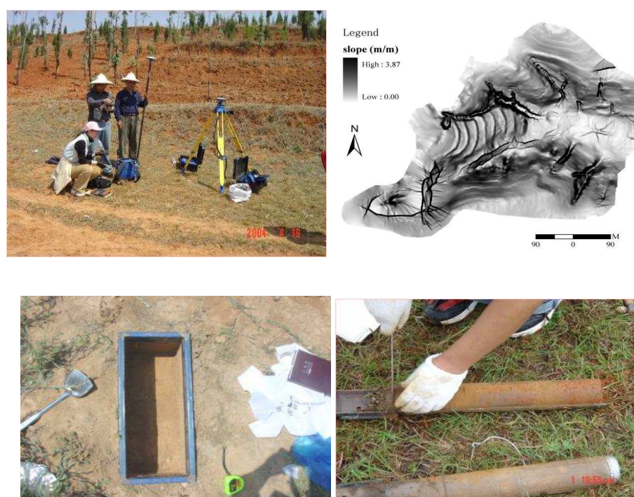
FIG. 5. GPS survey and soil sampling with core and scraper plate in Majiasongpo catchment of Xichang, SW China.
