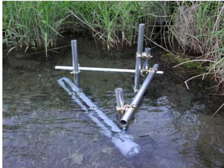
FIG.2. Suspended sediment sampler set in the stream at the outlet of the watershed.
