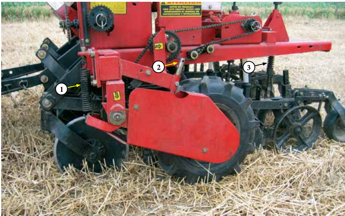
Figure 17. Penetration/depth control mechanism: 1. Pressure spring for cutting disk and fertilizer depth; 2. Limiting bolt of drive wheel; 3. Pressure spring for seed depth.
