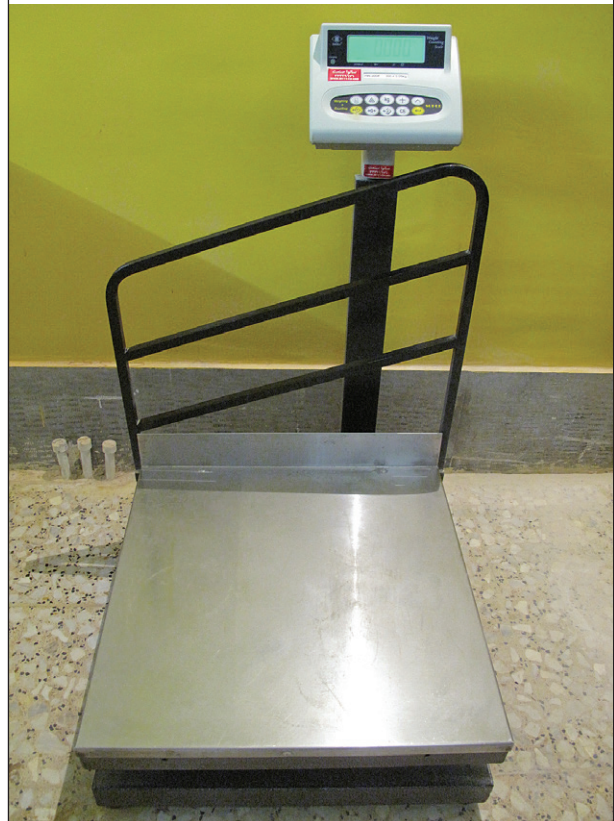
FIGURE 16 Scale properly placed and protected
