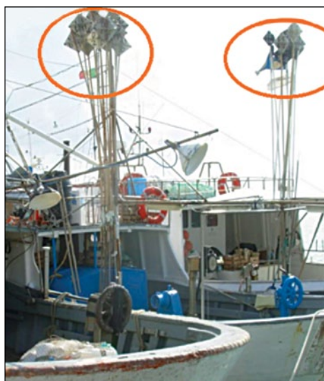
The presence of the radar reflectors indicate that the vessels are using the drifting longlines.
