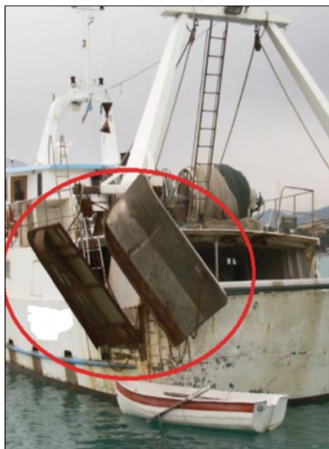
Two trawl doors are being used, which means that the vessel uses two different trawl nets.
