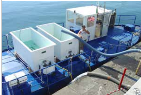
PLATE 102 Flushing out the last fingerlings at the farm site. Note the external slide mounted onto the tank's sluice and the red flexible tube mounted on the slide that extends into the cage
