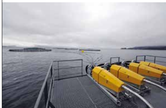
PLATE 113 Feed delivery pipes connecting the centralized feed system with the cages
