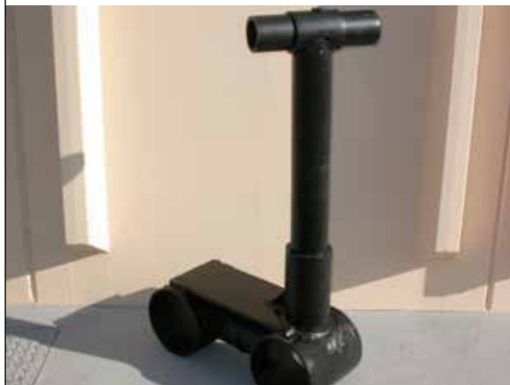
PLATE 23 HDPE bracket made with welded HDPE pipes, reinforced on the base of the stanchion
