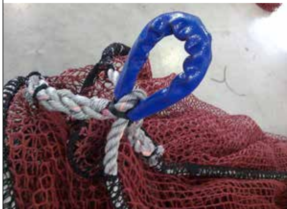
PLATE 64 Waterline rope loop with flexible pipe protection
