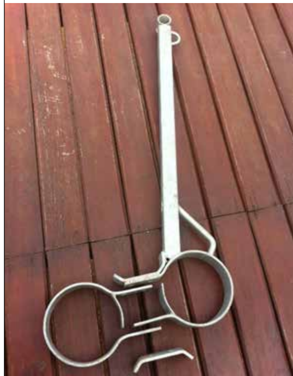
PLATE 28 Disassembled components of a galvanized steel bracket
