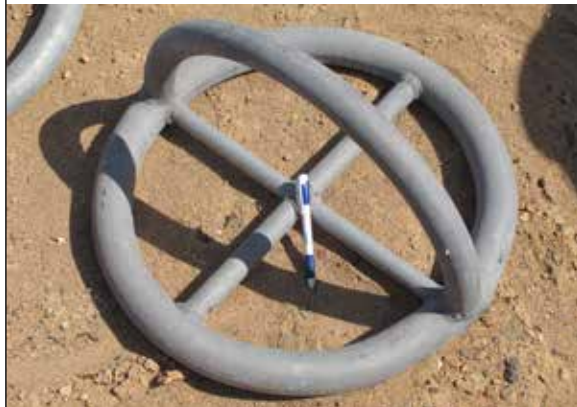
PLATE 19 Steel ring used as a corner plate. This component permits the rope to be knotted directly to the steel ring without using shackles
