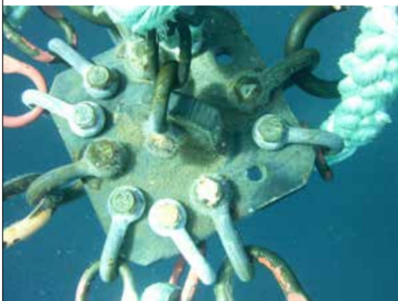
PLATE 13 Corner plate, 12 holes. Four are used to connect the main mooring lines; eight are used to connect the mooring bridles for the cages
