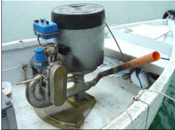
PLATE 104 Feed cannon with integrated air blower, powered by a petrol engine
