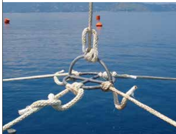
PLATE 21 Steel ring connected to grid lines and cage bridles
