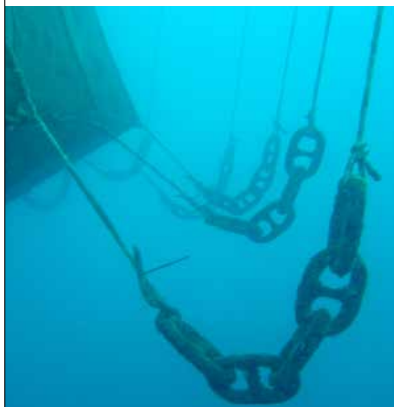
PLATE 34 Stud link chains used as sinkers. Chains are preferable for use as net tensioning ballasts because of the greater weight in water of steel, compared with concrete, stones or other materials
