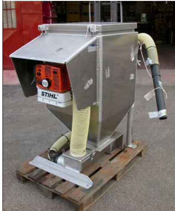
PLATE 105 Feed cannon with integrated air blower, powered by a petrol engine. In this case, the feed is transported to the blower through an electrically-powered auger (see Plate 106)
