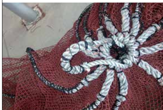
PLATE 67 Cross base ropes spliced on the central ring (with additional external loop)
