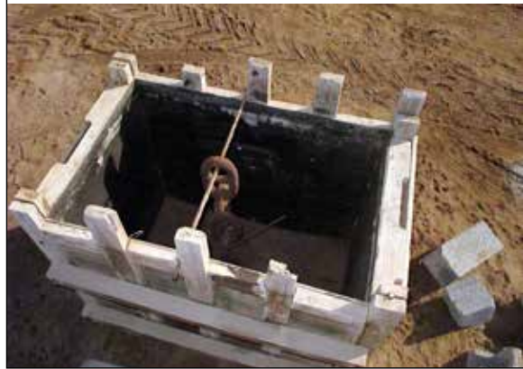
PLATE 5 Wooden mould ("form") for building concrete blocks in the field
