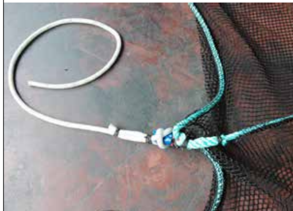
PLATE 63 Top loop with spliced tie rope
