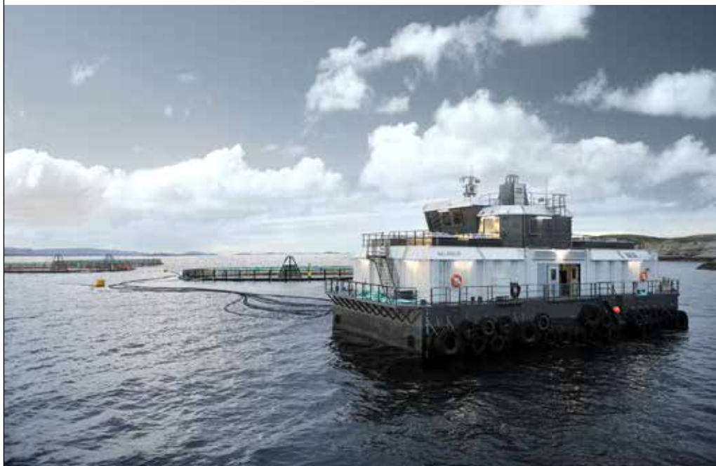
Centralized feed system on a purposely built barge
