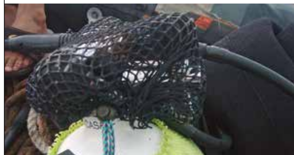
PLATE 124 A protective cover made of knotless netting is wrapped around the first stage of a scuba diving regulator to reduce the risk of it becoming entangled in the seine net
