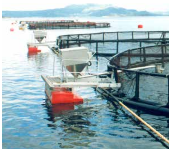
PLATE 113 Feed delivery pipes connecting the centralized feed system with the cages
