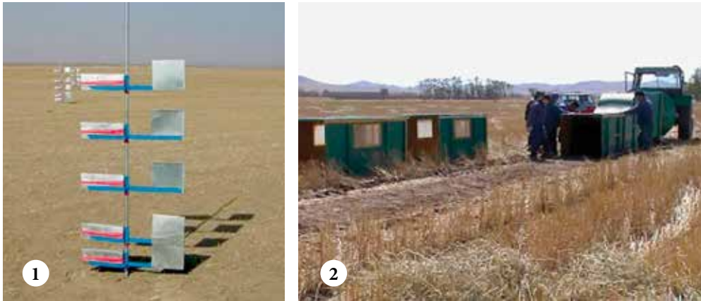
Figure 41. The big spring number eight dust sampler (1) and portable wind tunnel (2)
