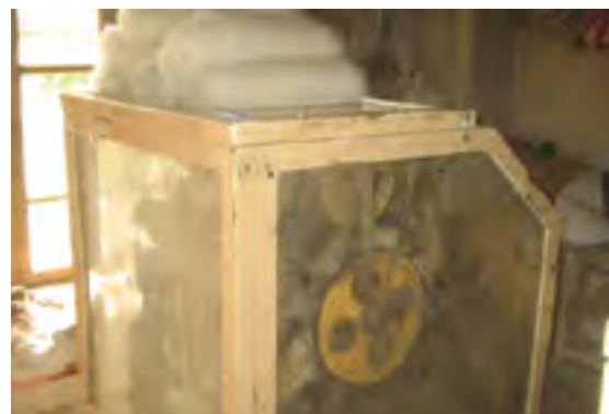
Figure 7: Special equipment for carding and scutching “fleece”, made in Russia, in a household in the village of Tapakurgan, Namangan region.
