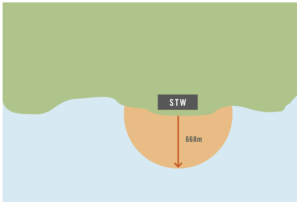
FIGURE A10.4 EXAMPLE OF A BUFFER ZONE BASED ON A SIMPLE DILUTION CALCULATION.
