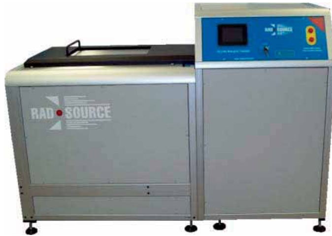
Figure 1.2a. RS-2400 self-shielded X-ray irradiator (Produced by RAD Source Technologies Inc., USA) in the Entomology Unit - Seibersdorf Laboratories - Joint FAO/IAEA - Programme of Nuclear Techniques in Food and Agriculture, Vienna, Austria (Mehta and Parker, 2011).
