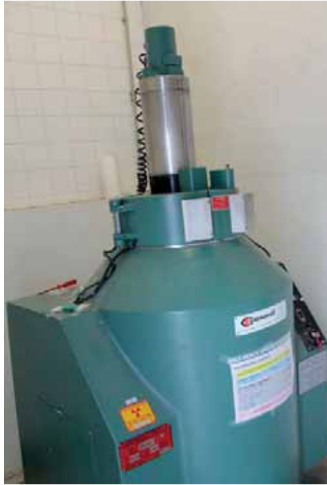
Figure 1.3a. Gamma-rays machine in the Joint FAO/IAEA Plant Breeding and Genetics Laboratory, Seibersdorf – Austria. Courtesy of M. Matijevic.
