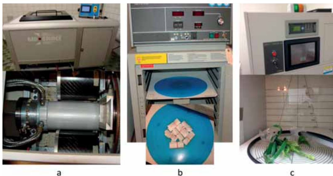
Figure 1.8. Representative X-ray machines; a) vertical rotating Rad Source RS2400 showing the machine (upper) and the sample chamber with the upper most Canister removed for ease view, b) Faxitron 650 (Faxitron bioptics LLC, Tuscon, AZ, USA) showing horizontally rotating tray with seed bag samples placed in the centre, and c) Hitachi Standard MBR-1520R-3 machine showing the sample chamber at the lower most position with green wheat spikes ready for irradiation. Courtesy of A. Mukhtar Ali Ghanim.
