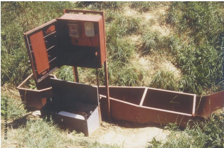
Figure 2.5. Example of Parshal fume used for measurements of suspended sediment (Lukacovce, Slovakia).
