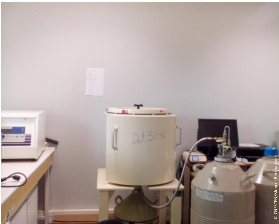
Figure 5.1. Laboratory gamma detector in lead shield and with nitrogen cooling (CNESTEN, Morocco).
