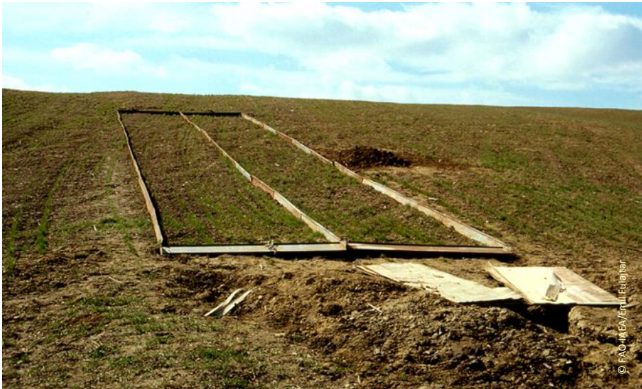
Figure 2.4. Example of erosion plots with total collection of sediment (Osikov, Slovakia).
