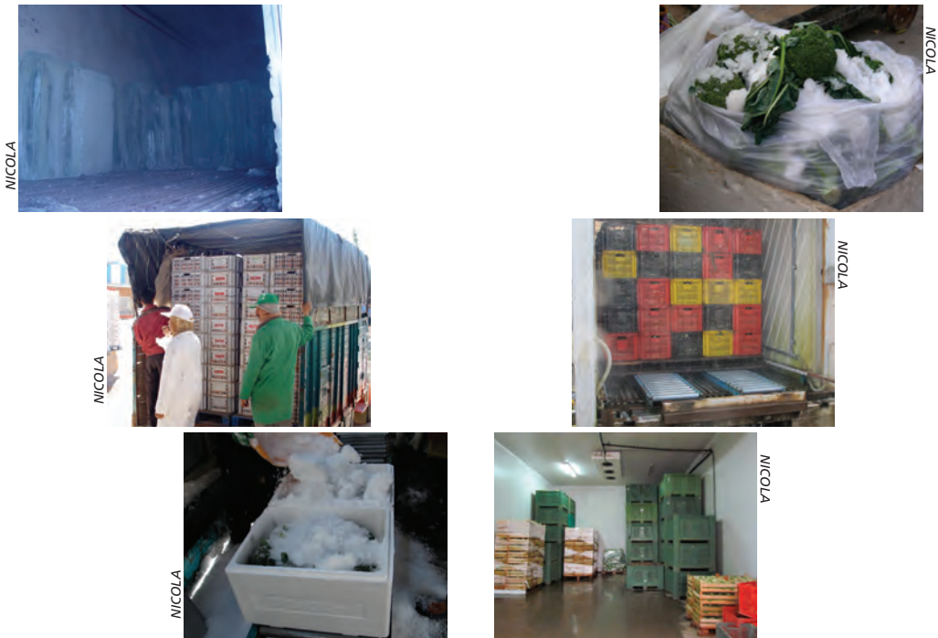
Plate 7 (From left to right and top to bottom) Truck with ice for transport from field to storage Body icing in closed box storage for rapid raw material cooling Closed and shaded truck for transport from harvesting area to storage Hydrocooling system in transport truck on arrival at packing house Top icing in closed insulated box storage for cold preservation of raw material before dispatching Storage room at cold temperature on a small farm in Croatia
