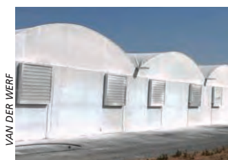
Plate 1 Shading by whitening of the greenhouse cover
