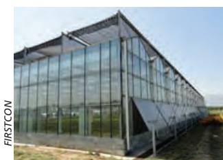
Plate 2 External shading net above the cover
